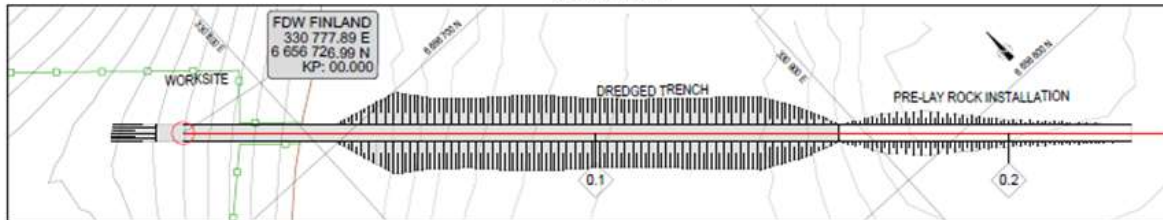
PULL-IN TRENCH GENERAL ARRANGEMENT SCALE 1:1000
