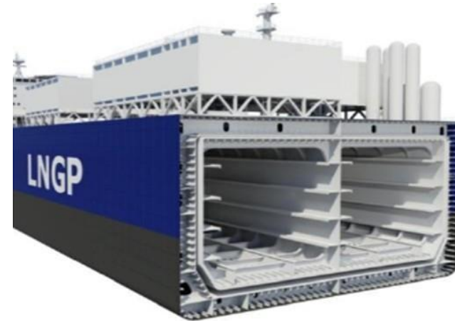
SPB tank application of Ni steel. Source: Flex LNG
